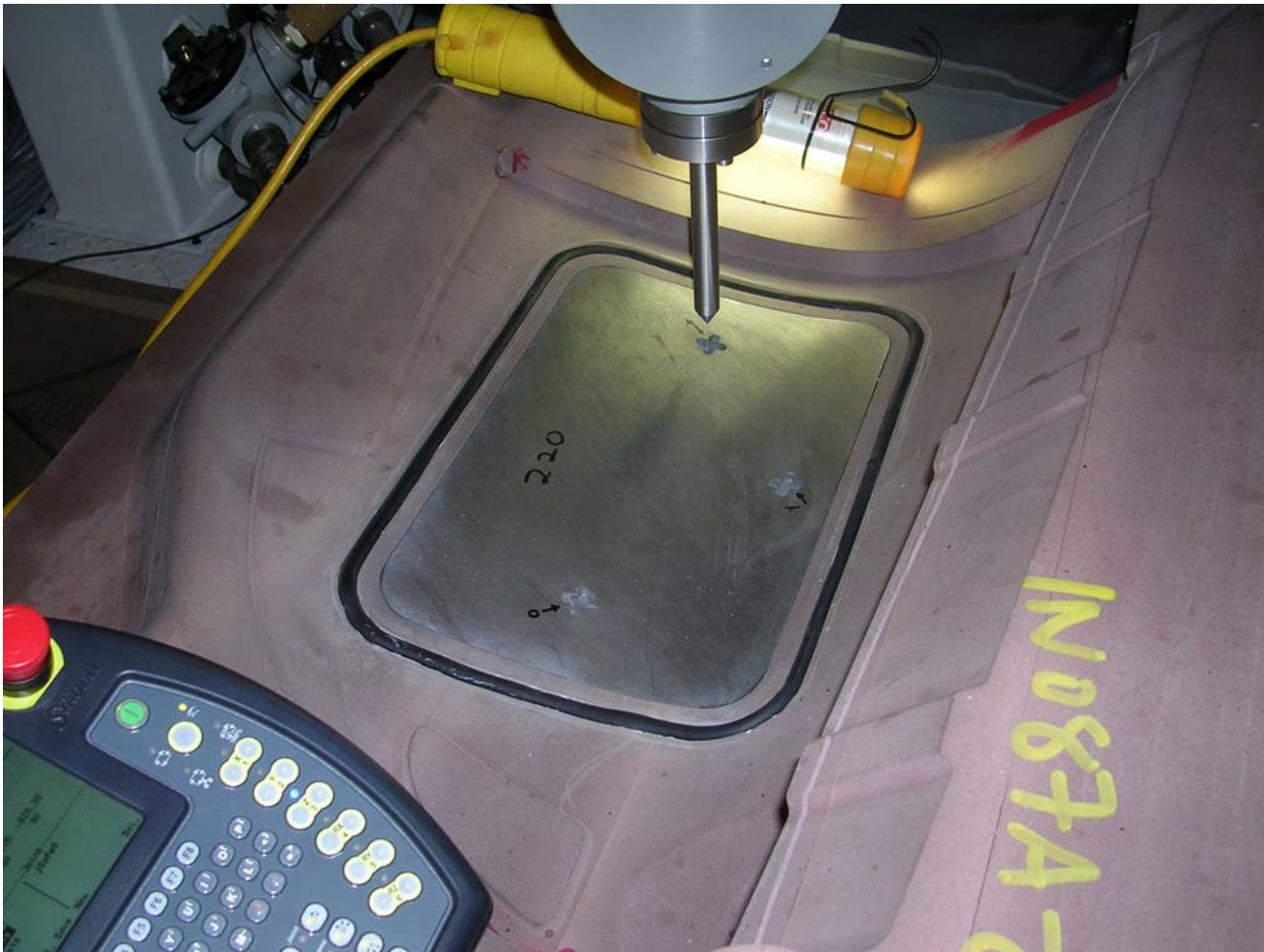
FIGURE 1: Intier Job# IN-068A (J61J) Scoring Fixture. Figure shows robot with precision pointer attached, teaching Fixture Coordinate System points. The Fixture Insert was designed to have three locating features machined into it to be used at teaching points.
