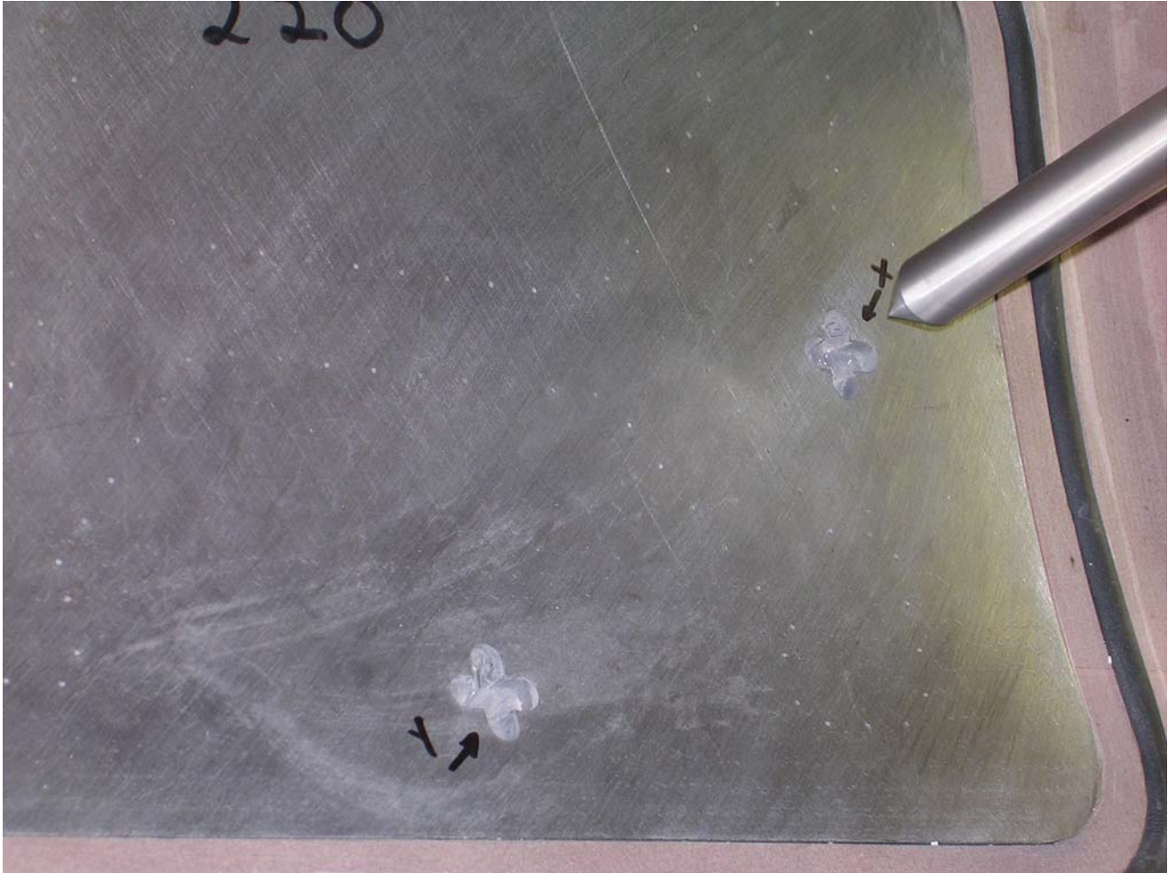
FIGURE 3: Closeup of cruciform features. One of the corner points of each feature is arbitrarily selected and used to teach a Fixture Coordinate System point.
